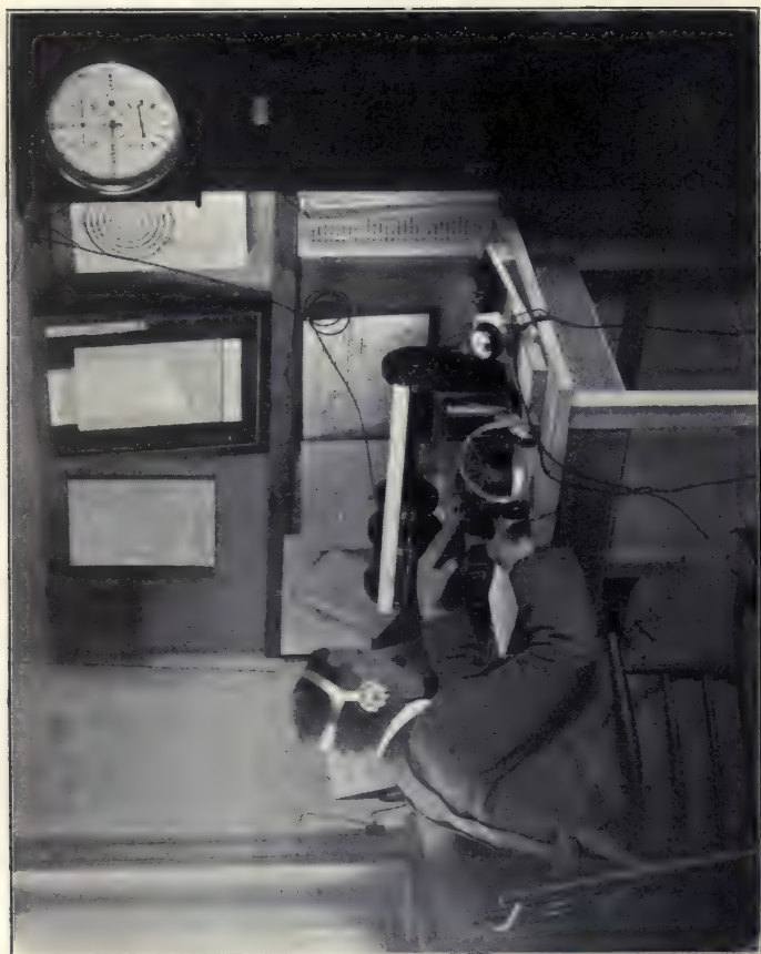
Fig. 9. —Apparatus for receiving Wireless Time and Weather Signals.
